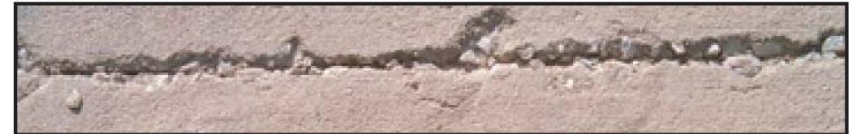
Figure 8-23. Close-up of different degrees of raveling caused by joint sawing (ACPA)
