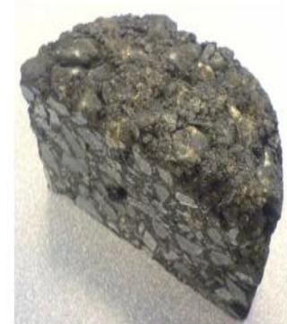
Mix manufactured with microalgae oil, using oedometric compaction system.
